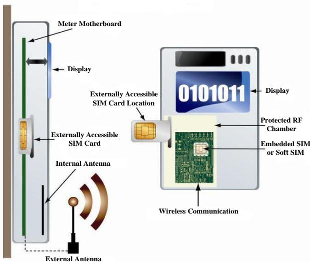
Fig. 3. The internal structure of a smart metering
