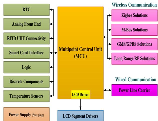
Fig. 4. Diagram block of the AMR network
