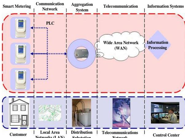
Fig. 2. Components of AMI Systems Network Architecture
