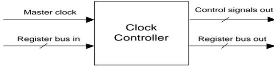
Figure 7. Describing Clock Controller signals
