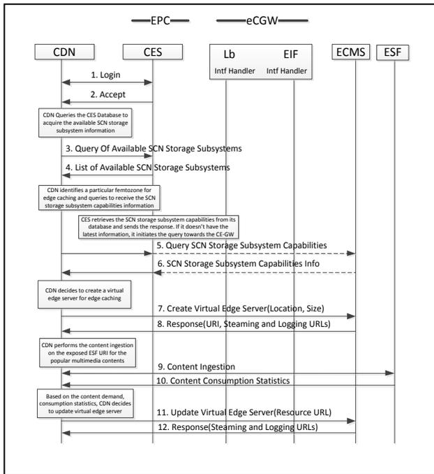
Figure 4. Managed Edge Caching Procedures
