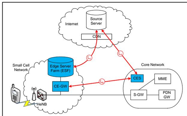
Figure 1. Managed Edge Caching Architecture
