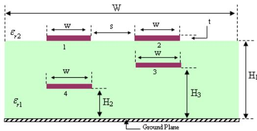
Figure 2. Cross section of unshielded four-conductor transmission lines.
