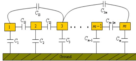
Figure 1. The per-unit length capacitances of a general m-conductor transmission line.
