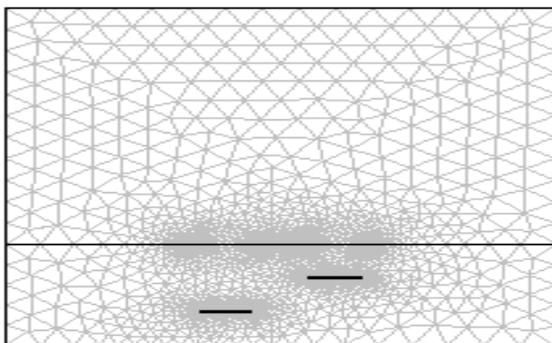
Figure 3. Mesh plot of unshielded four-conductor transmission lines.
