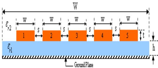
Figure 6. Cross section of unshielded five-conductor transmission lines.
