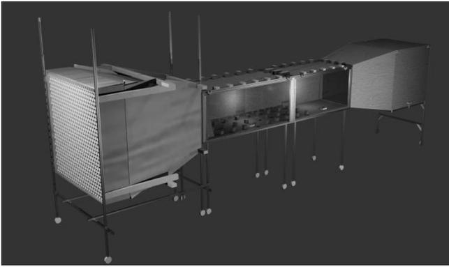
**Figure 6: Full Wind Tunnel Rendering, assembled by collaborating Team 1, Team 2 and Team 3 members**
