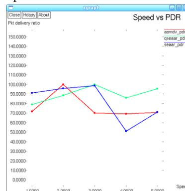
Fig 4.10 Comparison of packet delivery ratio versus speed
