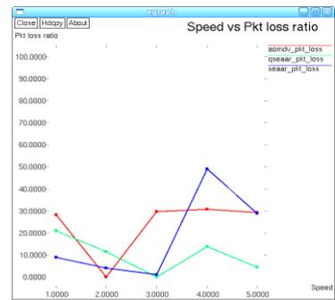
4.6 Comparison of packet loss ratio versus speed
