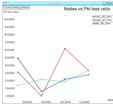
Fig 4.1 Comparison of packet loss ratio versus nodes
