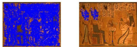
Figure 13: Detection results for the image in Figure 12 with all keypoints detected (left) and output image with valid matching keypoint (right).
