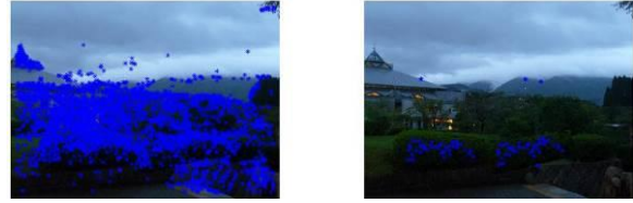
Figure 19: Detection results for the image in Figure 18 with all keypoints detected (left) and output image with valid matching keypoints (right).
