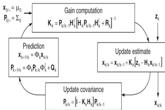
Figure 1. Operation of Kalman filter
