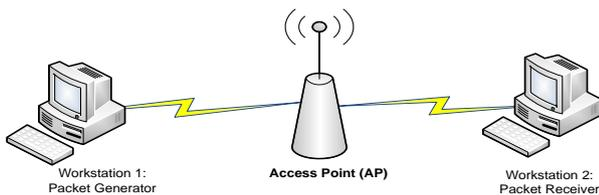
**Figure 1: Network test-bed for Windows XP, Windows 7 and Fedora 12**
