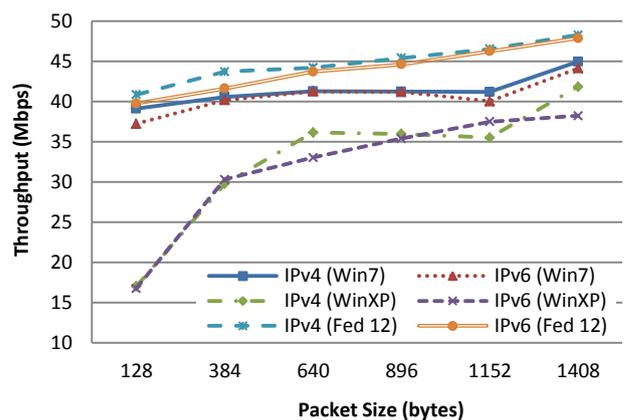
Figure 2: TCP Throughput of Windows and Fedora 12 Operating Systems for 802.11n (open systems)
