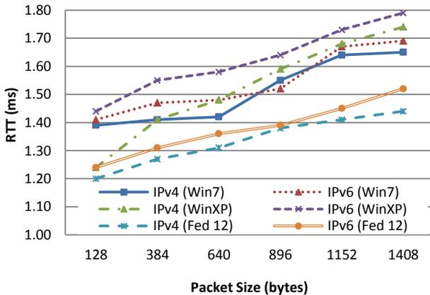
Figure 4: TCP RTT of Windows and Fedora 12 Operating Systems for 802.11n (open systems)
