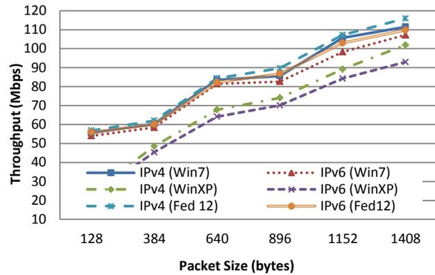
Figure 3: UDP Throughput of Windows and Fedora 12 Operating Systems for 802.11n (open systems)
