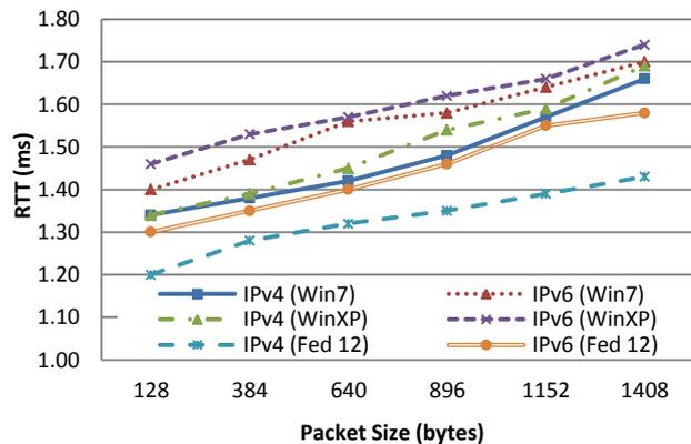
Figure 5: UDP RTT of Windows and Fedora 12 Operating Systems for 802.11n (open systems)
