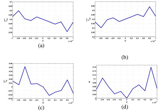
Figure 3: Effect of lens distortion on means of local shading measures: (a)  $\overline{I_{xx}}$ , (b)  $\overline{I_{yy}}$ , (c)  $\overline{I_{xy}}$ , (d) Error  $\varepsilon_\kappa$  versus  $\kappa$ .
