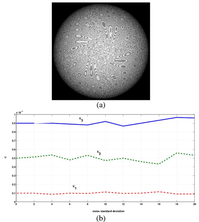
Figure 5: Proposed method performance versus noise: (a) Input synthetic textured sphere image. (b) The estimated lens distortion coefficient  $\kappa$  versus noise standard deviation for 3 ground truth values ( $1 \times 10^{-6}$ ,  $5 \times 10^{-6}$ , and  $9 \times 10^{-6}$ ).
