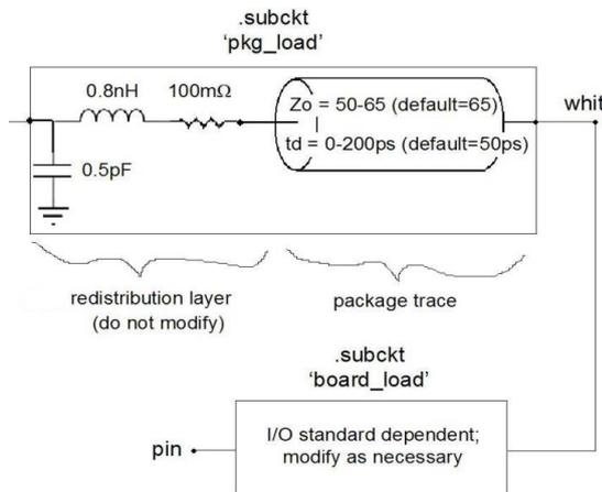
Fig. 7. Package parasitics of FPGA input/output buffer
