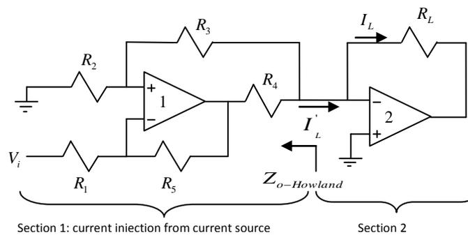
Figure 3. The new topology of current source designed.
