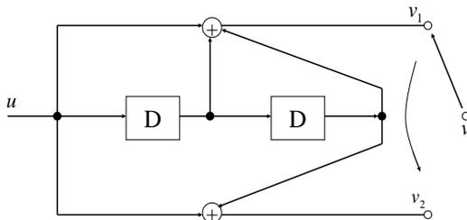
Figure 1. Encoder for the  $(2,1,2)$  convolutional code with generators  $g_1=(111)$  and  $g_2=(101)$
