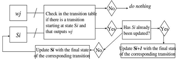
Figure 8. Functional description of the decoder's circuitry
