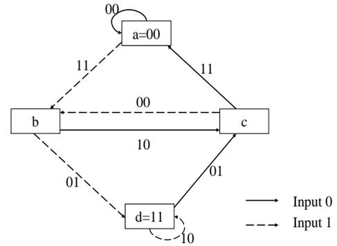
Figure 2. FSM for the encoder of figure 1
