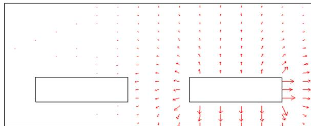
Figure 5. Streamline plot of shielded two-strip conductors in a homogenous medium
