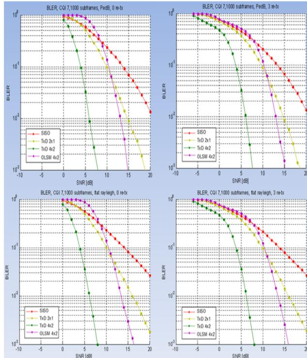
**Figure 2. BLER vs SNR for 1000 Subframes with 0 and 3 re-tx:
