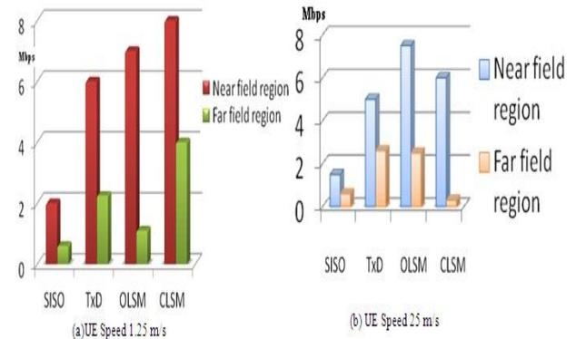
Figure 7. Throughput with Changed Speed for Transmission Modes
