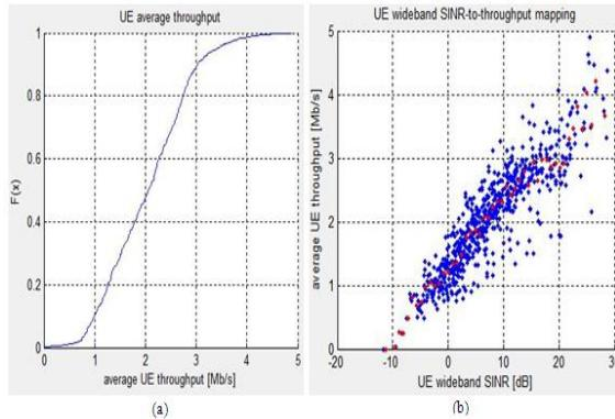
**Figure 4. UE Wideband SINR to Throughput Mapping**
