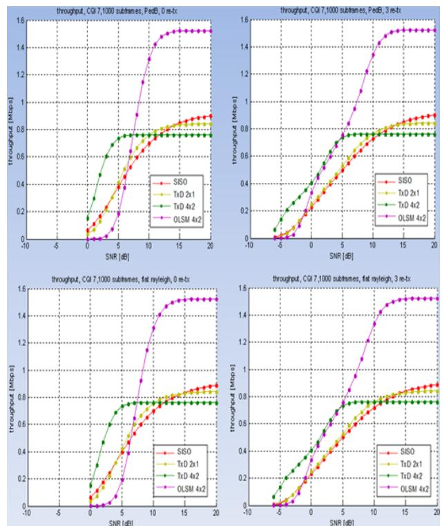
Figure 1. Throughput vs SNR for 1000 Subframes with 0 and 3 re-tx: PedB channel (top) & flat rayleigh channel (bottom)
