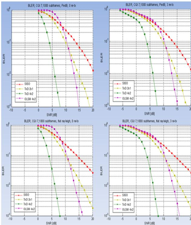
Figure 2. BLER vs SNR for 1000 Subframes with 0 and 3 re-tx: PedB channel (top) & flat rayleigh channel (bottom)
