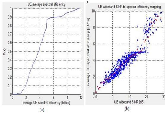
**Figure 5. UE Wideband SINR to Spectral Efficiency Mapping**
