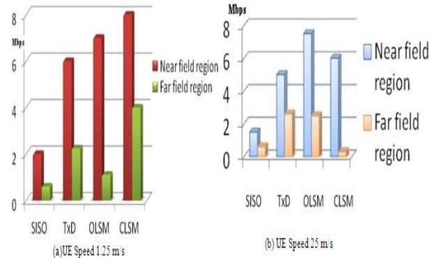
**Figure 7. Throughput with Changed Speed for Transmission Modes**
